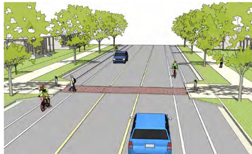
Street after Road Diet: addition of bicycle lanes, reduces four travel lanes to two travel lanes and one turning lane
